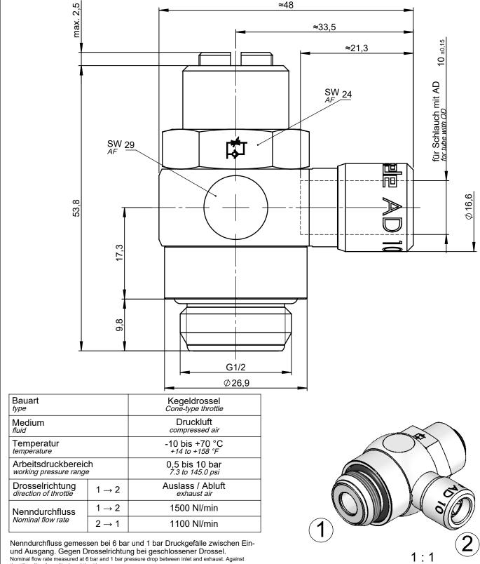
Nominal flow rate measured at 6 bar and 1 bar pressure drop between inlet and exhaust. Against throttling direction with closed throttle.
